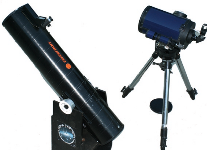
Fig. 4.2. Newtonian ( left ) and Schmidt-Cassegrain ( right ) telescopes. Note how much shorter the Schmidt-Cassegrain telescope is compared to the Newtonian. The Newtonian is on a Dobsonian mount and the Schmidt-Cassegrain is on an equatorial mount (credit: Truman Boyle).
