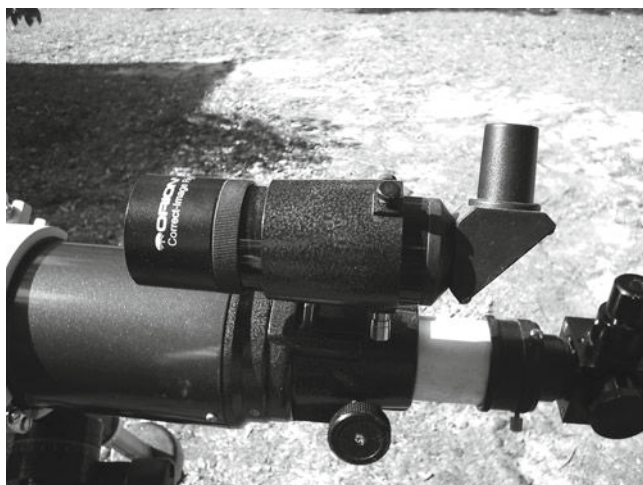
Fig. 4.21. A right angle finder on a telescope with a star diagonal (credit: Richard W. Schmude, Jr.).
