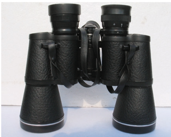
Fig. 3.3. Porro prism binoculars. Note that the eyepieces are not directly behind the larger objective lenses (credit: Richard W. Schmude, Jr.).
