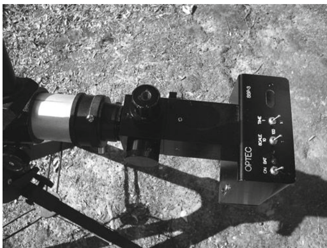
Fig. 4.42. An SSP-3 photometer inserted into the 1¼ inch eyepiece hole of a telescope (credit: Richard W. Schmude, Jr.).
