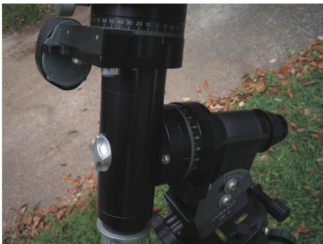
Fig. 4.6. Setting circles on a German equatorial mount (credit: Richard W. Schmude, Jr.).
