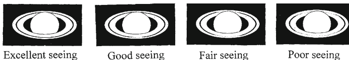
Fig. 4.23. If Saturn's rings are tilted then one can estimate the seeing by looking at Cassini's division, which is the dark band in the rings. If Cassini's division can be seen to the edge of Saturn then the seeing is excellent (credit: Richard W. Schmude, Jr.).
