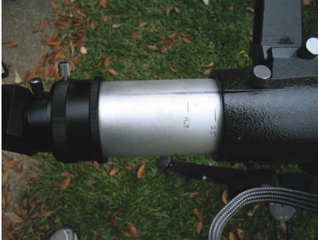
Fig. 4.11. An image showing marks on the drawtube where my 25 and 9.7 mm eyepiece come into focus. I move the drawtube until it lines up with the appropriate mark and the telescope is in focus (credit: Richard W. Schmude, Jr.).
