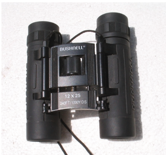
Fig. 3.2. Roof prism binoculars with a magnification of 12 and objective lenses with diameters of 25 mm (credit: Richard W. Schmude, Jr.).
