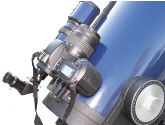
Fig. 4.35. The camera is on top of a telescope that tracks. This is known as a piggy-back arrangement (credit: Truman Boyle).
