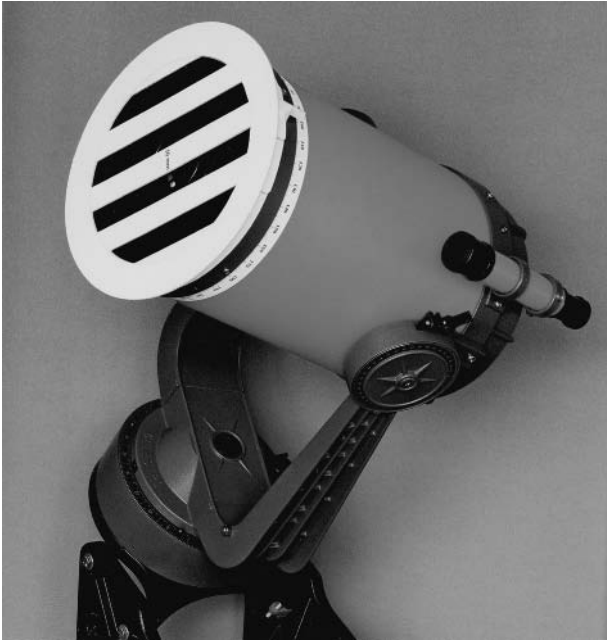
Figure 14.1. The author's 20-cm Schmidt-Cassegrain equipped with a 50-mm grating. The first-order images are 2.3 arcseconds from the zero-order image. See also Figure 14.5a below. The position angles can be read on a 360° scale.
