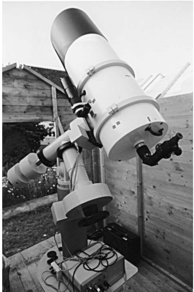
Figure 20.8. The 32.5-cm Cassegrain of Andreas Alzner fitted with a double image micrometer.
