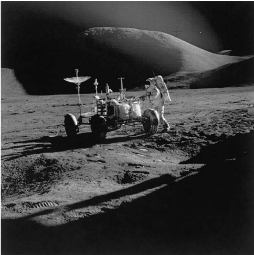
Fig. 2.1 Lunar rover The battery-powered lunar rovers, used in the last three Apollo missions, could carry two astronauts and all their equipment for kilometers across the lunar surface. The astronauts deployed instruments and returned rocks to the Lunar Module , which carried them back to their orbiting Command Module while the rover remained on the Moon. Because there is no substantial atmosphere, water or weather on the Moon, both the rover and the footprints in the lunar soil may last for millions of years. By that time micrometeorites will have pitted the rover and erased the footprints. (Courtesy of NASA.)
