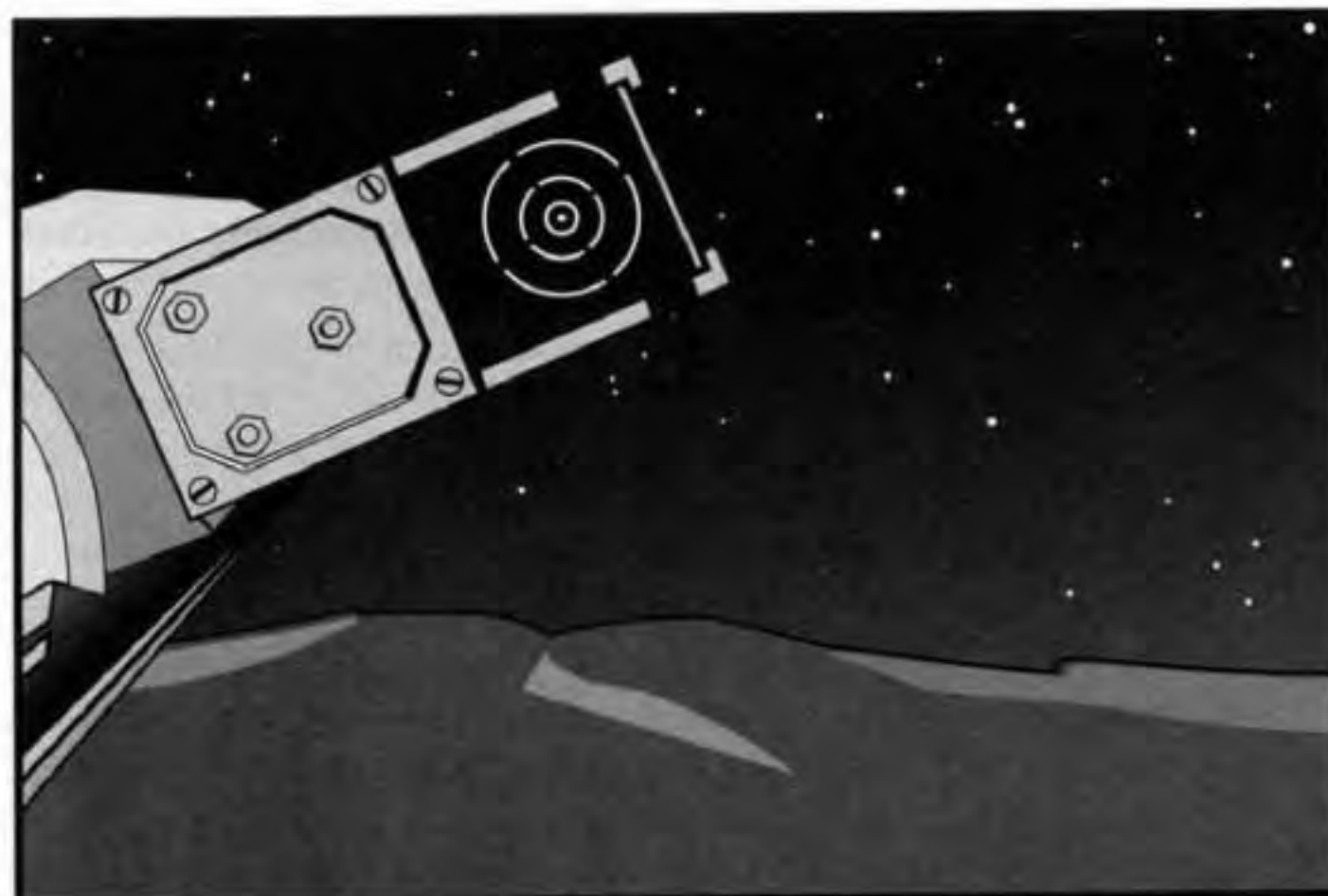
Figure 6-3 The Telrad sight rings are “projected” onto the sky. Unlike the traditional gunsight there is no parallax. Alignment is unaffected by how close the eye is placed to the Telrad. It’s used with both eyes open.
