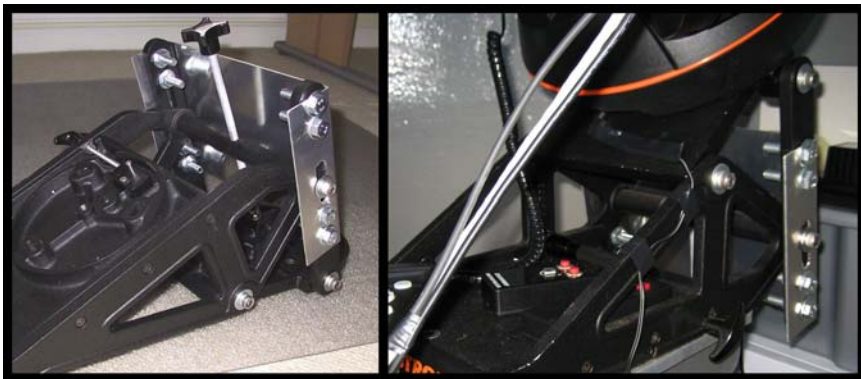
Figure 1.4. The modification made to the standard Celestron “heavy-duty” wedge. A 2mm thick aluminium sheet is used to close off the open-ended box section of the wedge. Right-hand photo, the wedge in-situ.
