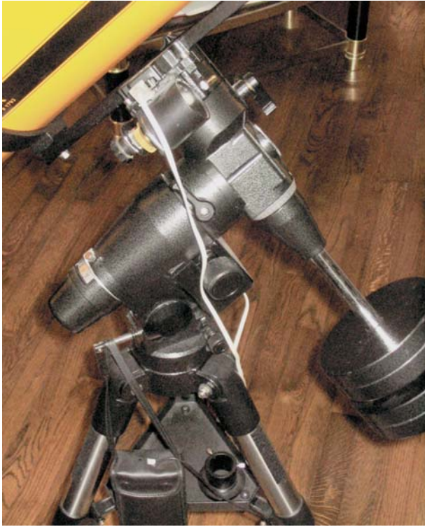
Plate 5. The ubiquitous Synta EQ4 German Equatorial Mount.
