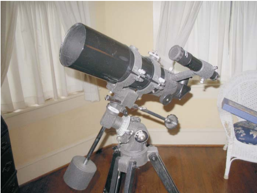
Plate 2. Celestron's 80 mm f/5 refractor.
