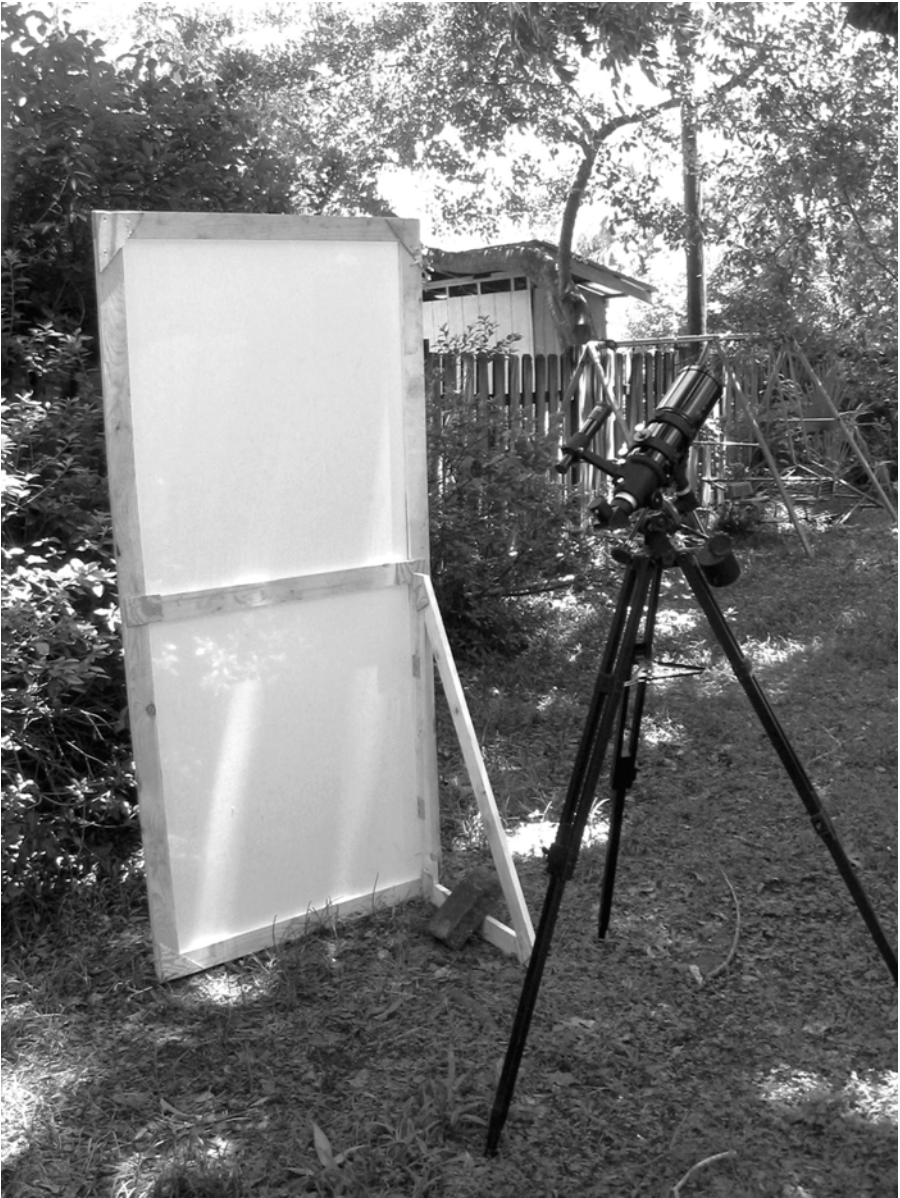
Plate 14. Stage flat light shield (unpainted to show detail).
