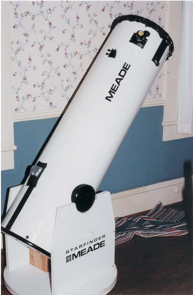
Plate 3. Meade's inexpensive but effective 12.5 inch Dobsonian.
