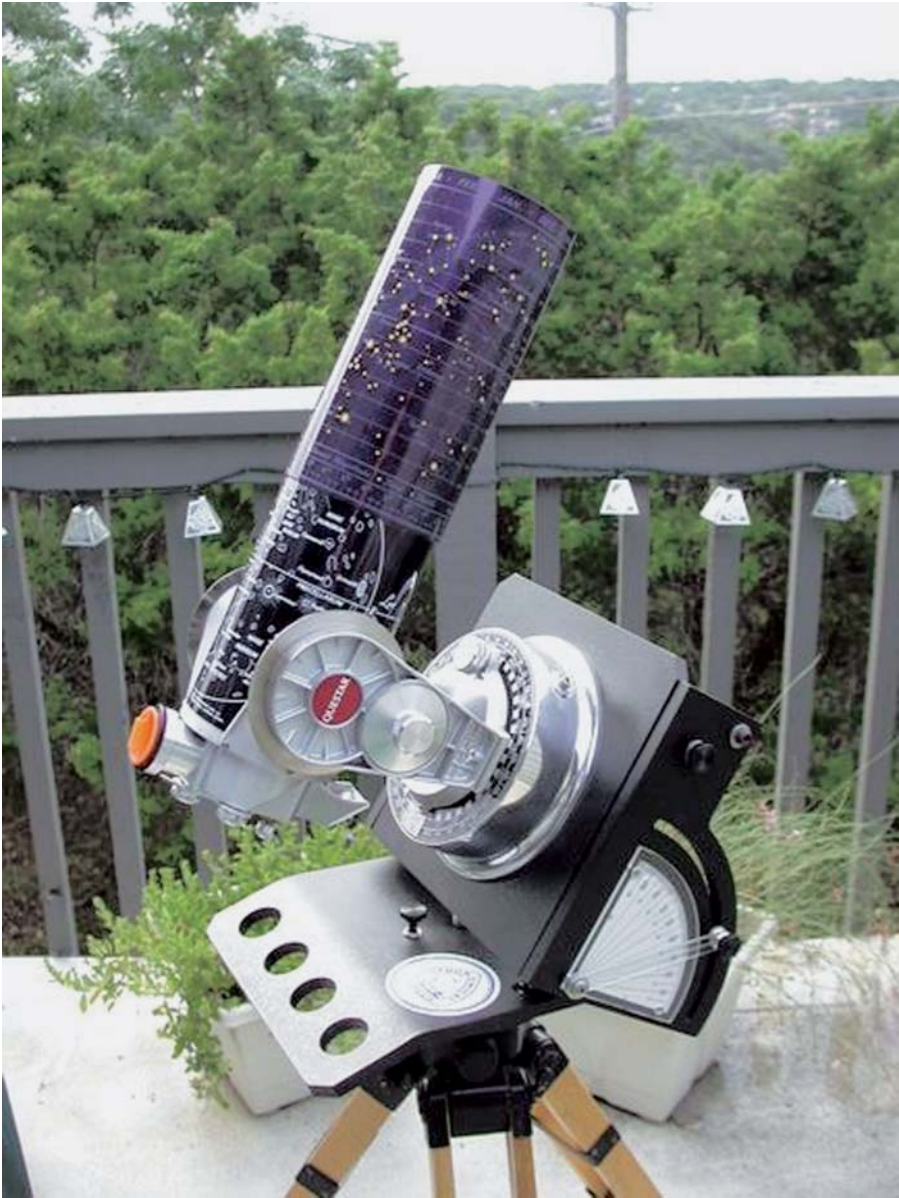
Plate 8. The beautiful Questar 3.5 Maksutov Cassegrain Telescope. (Courtesy of Jack Estes)
