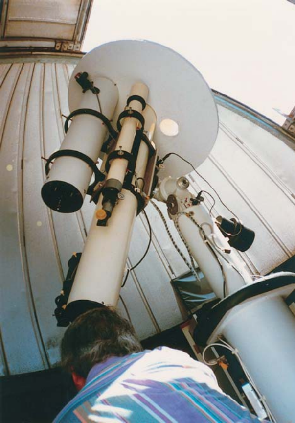
Figure 11.3. The author at the working end of a 6-inch refractor equipped with a hydrogen-alpha solar filter. Note the circular disk at the top of the tube (through which the filtered objective end of the telescope itself protrudes) covering both the finder and an auxiliary short-focus reflector (a very important precaution!). This also serves to block direct sunlight from falling on the observer. Photo by Sharon Mullaney.
