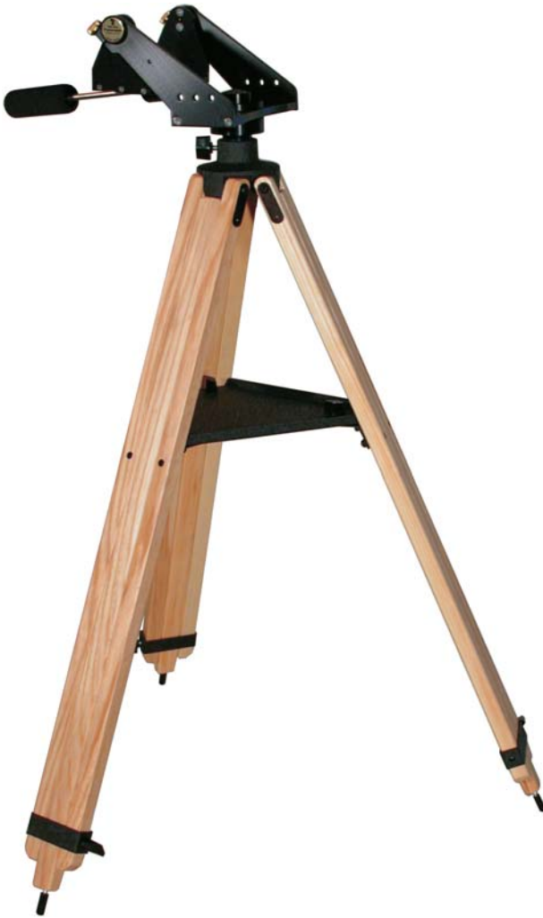
Figure 3.3. An extremely sturdy, well-made altazimuth fork mounting with wooden tripod legs (which are preferred over metal ones for damping vibrations). Courtesy of Tele Vue Optics.
