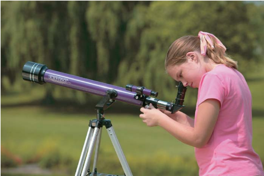
Figure 1.1. Given good optics, even a small telescope can provide a lifetime of celestial viewing pleasure for people of all ages. Shown here is the ubiquitous 2.4-inch (60mm) refractor, which has long been (and continues to be) the most common telescope in the world. Courtesy of Edmund Scientifics.
