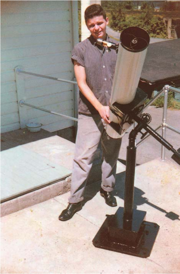
Figure 1.2. The author shown at the age of sixteen with his 6-inch equatorially mounted Newtonian reflector, entirely home-made (including its parabolic primary mirror). Today, most “telescope makers” opt for purchasing commercial optics and mounting them in an instrument of their own construction (typically as a Dobsonian reflector, especially for larger apertures). Photo by the author.
