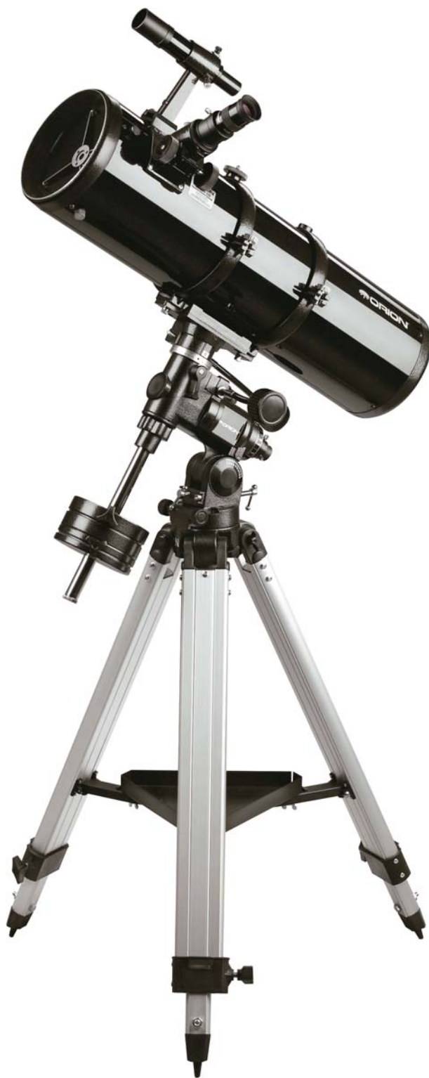
Figure 5.2. Orion's AstroView classical 6-inch Newtonian reflector, shown here on a German equatorial mount. The traditional focal ratio for a 6-inch, long preferred by telescope makers and observers, was (and for many still is) f/8 . But in a bid to make telescopes more compact and portable, shorter ones have appeared on today's market – as in this case, which is an f/5 system. Courtesy of Orion Telescopes & Binoculars.
