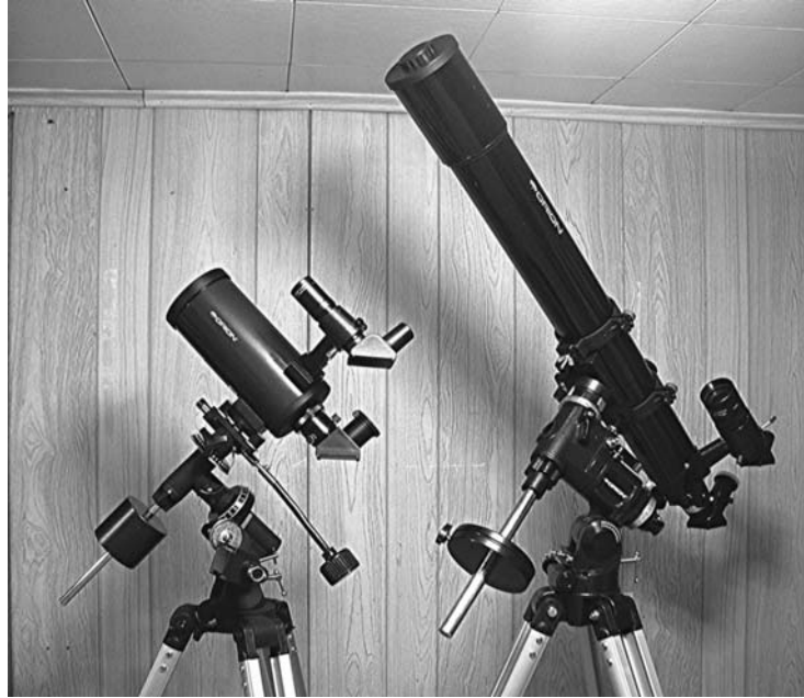
Figure 3.1. A comparison of German-type equatorial mounts.
