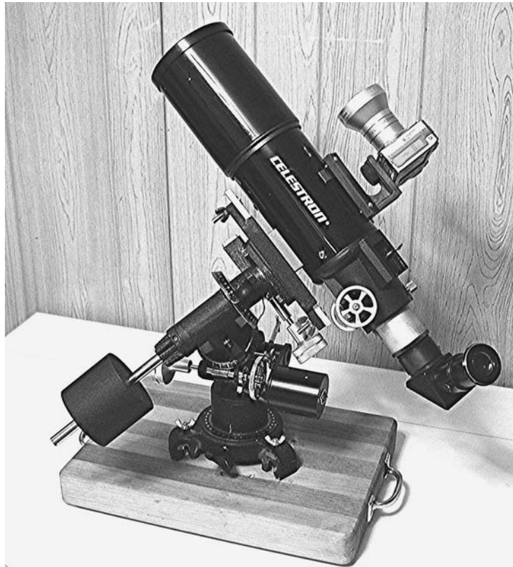
Figure 5.3. A digital camera with a telephoto adapter mounted on an 80-mm f/5 refractor.
