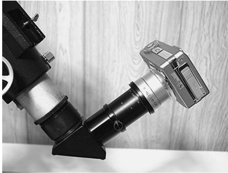
Figure 5.2. A digital camera with an afocal adapter on a 25-mm eyepiece.
