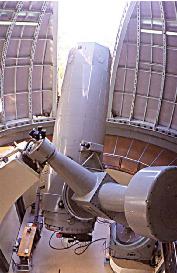
Fig. 1.7 The 193-cm telescope at the Observatoire de Haute Provence. Equipped with the high-resolution Elodie spectrograph, it enabled the first exoplanet orbiting a solar-type star, 51 Peg, to be discovered in 1995
