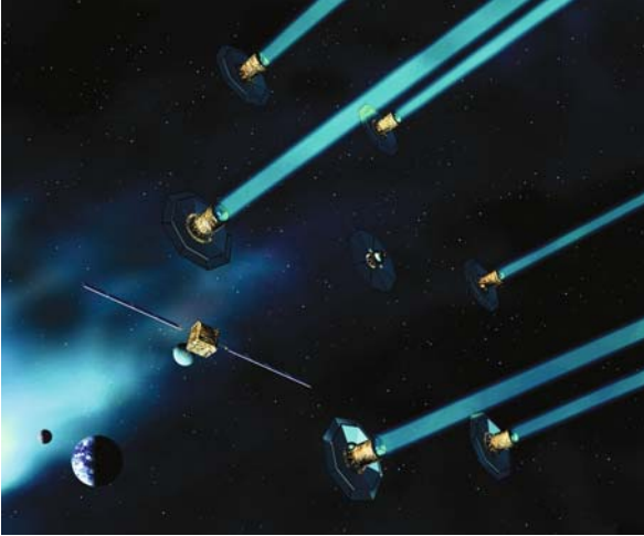
Fig. 8.25 Artist's impression of the DARWIN mission, where six telescopes are arranged in a circle. The central satellite is the recombination laboratory. An eighth satellite, not shown here, handles transmission of information to Earth and monitors the spacing of the overall array (image credit: courtesy ESA)
