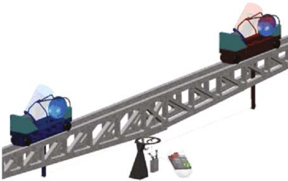
Fig. 8.24 Artist's impression of the ALADDIN instrument. The two dark-fringe recombination telescopes are mobile along a rail, the orientation of which may also be changed (Alcatel Alenia Space)
