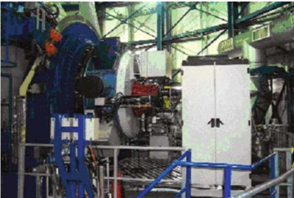
Fig. 8.16 The NAOS instrument and the CONICA camera at the Nasmyth focus of Yepun, one of the four 8.2-m telescopes of the VLT on Mount Paranal in Chile (ESO image)
